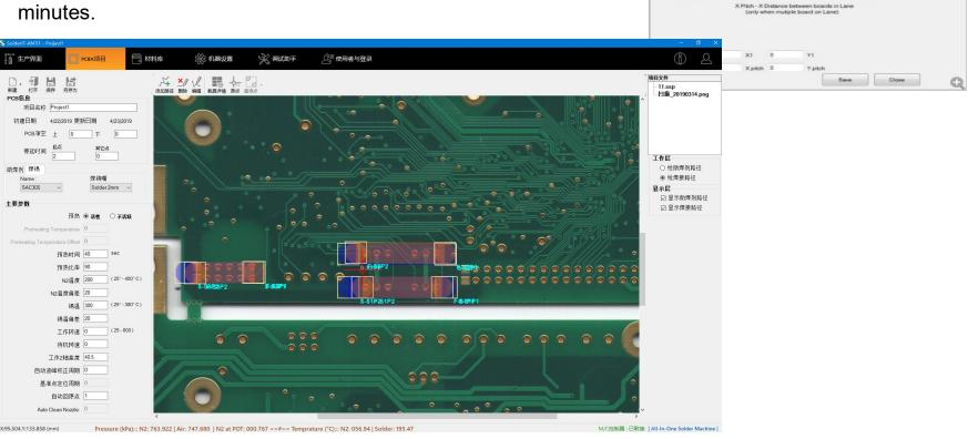
All motion path can be editable, include soldering speed, empty move speed, dwell time, solder Z height, wave height, wave slop speed etc.
