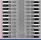
DIMM Connector Inspection
