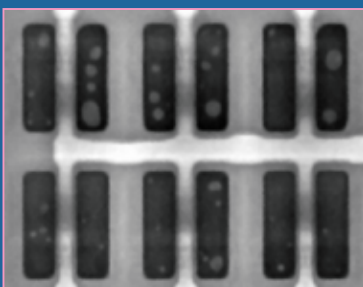
Void Inspection of LED
